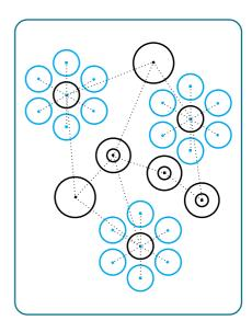
The Wave Relay<sup>TM</sup> system lets any device relay data over multi-hops between nodes.
